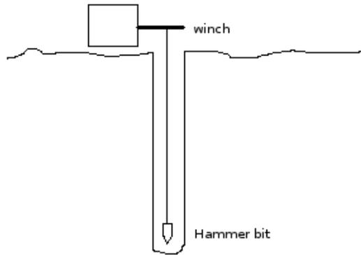
Figure 2: Cable tool drilling. The cable tool has a hammer type bit. This is raised with the winch and then allowed to fall and pulverize the rock. The cuttings are removed in a method similar to in auger drilling.
