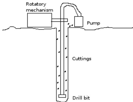
Figure 3: The whole drill pipe is rotated to drill through the rock. A fluid is pumped down the drill pipe and back up outside the drill pipe. The cuttings are carried up by this flow.
