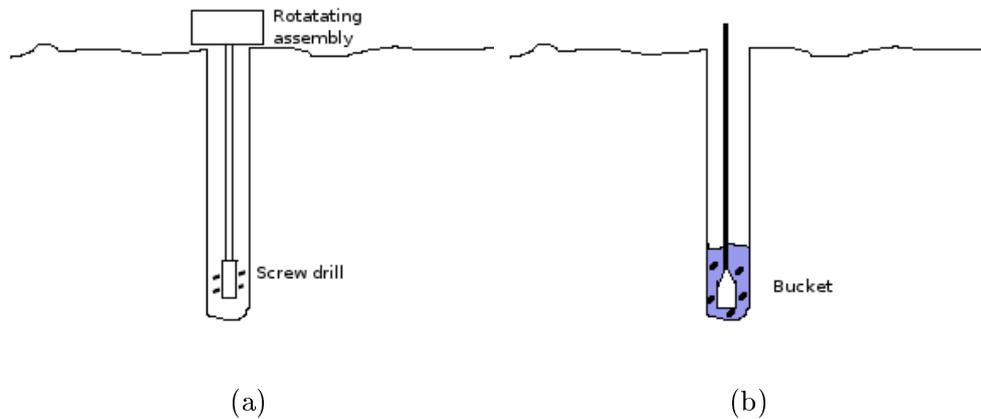
Figure 1: Auger method consists of alternatively drilling with a screw and removing cuttings with a bucket. The bucket has a flap on the bottom that opens up when it hits the water. As the bucket is filled, the flap closes and the bucket can be pulled out.
